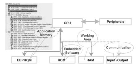
Fig. 1. Microprocessor card architecture
