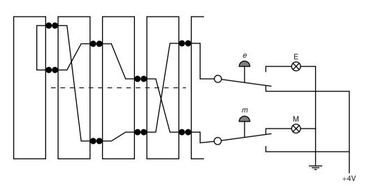
Fig. 1. Electric current through a three-rotor Enigma
