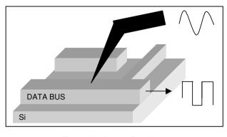
Fig. 4. Mechanical probing
