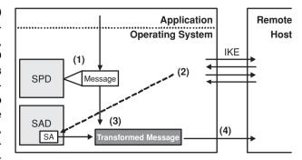
Fig. 1. IPsec packet processing
