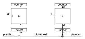
Fig. 4. The m-bit CTR mode of an n-bit block cipher
