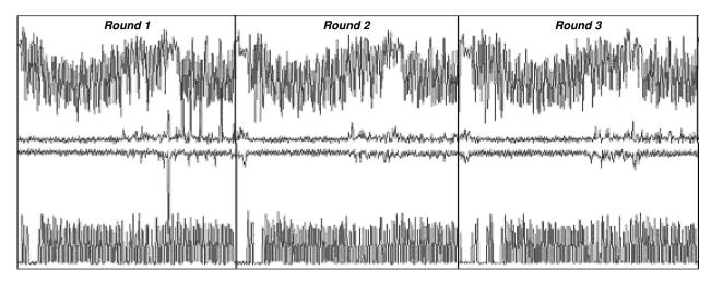
Fig. 7. DPA trace of the three first rounds of DES (two upper (respectively lower) curves: power consumption curve of maxima (respectively minima) of a single execution and DPA curve of maxima (respectively minima))
