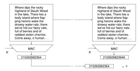
Fig. 1. Using a MAC algorithm for data authentication
