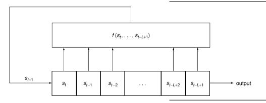
**EXAMPLE.** Let us consider L=3 and let the *feed-back function*  $f(s_t,s_{t-1},s_{t-2})=s_t\cdot s_{t-1}+s_t+s_{t-2}$  (in its algebraic normal form, with binary operations "·"-AND and "+"-XOR) be given by the following truth table:
