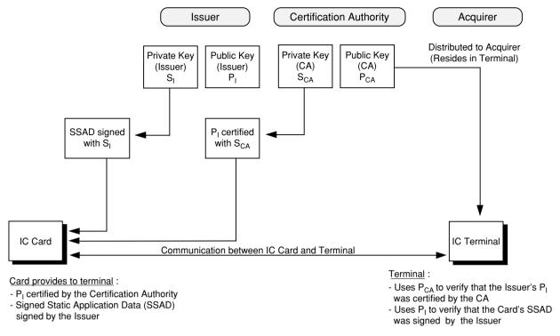
Fig. 2. Diagram of static data authentication
