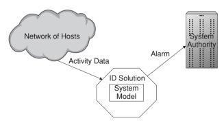
Fig. 1. Intrusion detection techniques compare environmental state (e.g., activity data) with a model of normal or anomalous system behavior
