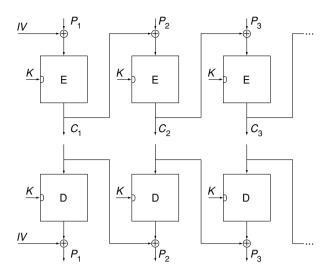
Fig. 2. The CBC mode of a block cipher
