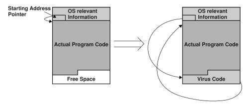
Fig. 1. How a virus attaches itself to a binary executable
