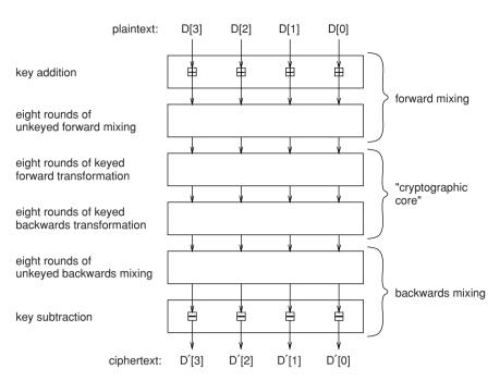
Fig. 1. High-level structure of MARS
