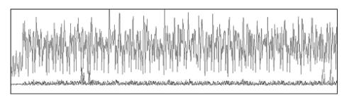
Fig. 4. Bit tracing (upper curve: power consumption of a single execution; two lower curves: DPA curves respectively tracing the first and last data bit of a targetted process)
