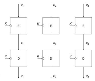
Fig. 1. The ECB mode of a block cipher
