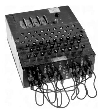
Fig. 2. Cipher machine Enigma (four-rotor version)
