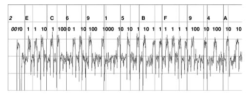
Fig. 6. SPA trace of the basic square-and-multiply algorithm
