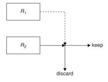
**EXAMPLE.** Let us consider  $R_1$  of length three, with the feedback relation  $s_{t+1} = s_t + s_{t-2}$ , and  $R_2$  of lenth four, with the feedback relation  $s_{t+1} = s_t + s_{t-3}$ . Then the following happens (the
