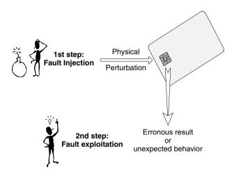
second step consists in exploiting the erroneous result or unexpected behavior. Fault exploitation depends on the software design and implementation. In the case of an algorithm it will also depend on its specification since the fault exploitation will be combined with cryptanalysis most of the time. Depending on the type of analysis performed, the fault injection will have to be done at a precise instant or roughly in a given period of time.
