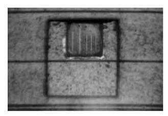
Fig. 2. Example of window opened in the passivation layer using laser cutter
