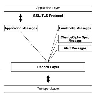
Fig. 1. SSL layer and message structure
