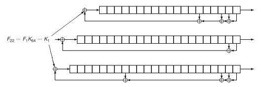
Fig. 1. Initialization of the A5/1 running-key generator
